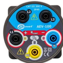
**Riso+ / Rcont+ / H / L1** – insulation resistance measurement / continuity measurement / earth resistance measurement / connection to the phase conductor of the tested object.
